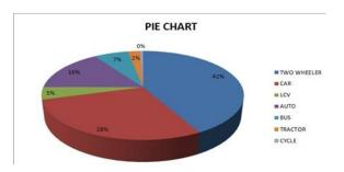
Similar survey Traffic Volume Count were conducted at Bannerghatta Road at different timings i.e., morning, evening, peak hours. Method of volume study can be done in two ways, Automatically and. Manually. Here survey was conducted manually.
