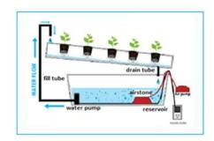
Fig-3: Nutrient Film System
