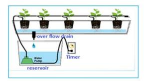
Fig-4: Continuous Drip System
