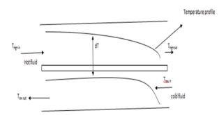
Figure: Temperature profile of hot and cold fluid when flown in opposite direction
