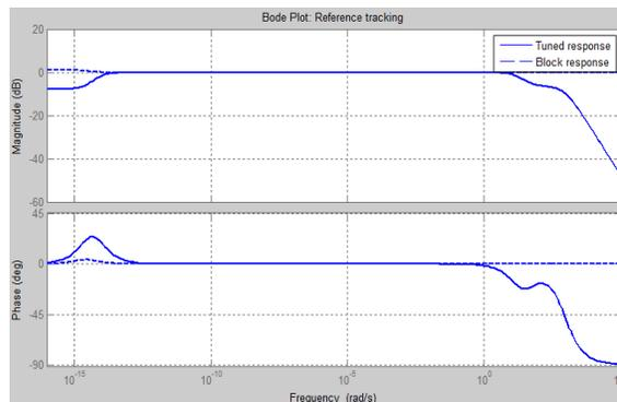
Fig. 12 CPSS-PID reference tracking on frequency graph for the CPSS
