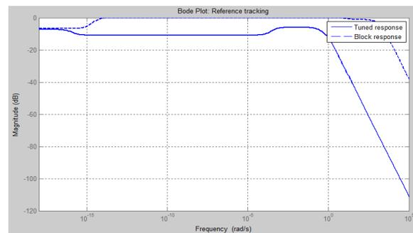
Fig. 21 Generic-PID reference tracking on frequency graph
