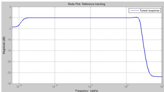
Fig. 15 PSO-PID reference tracking on frequency graph
