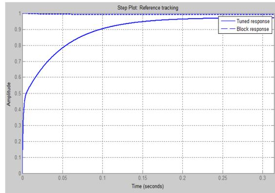
Fig. 11: CPSS-PID reference tracking on time graph
