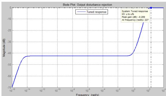
Fig. 16 PSO-PID output disturbance rejection
