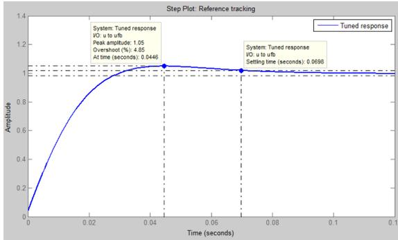
Fig. 14 PSO-PID reference tracking on time graph
