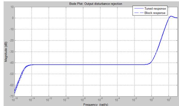
Figure 19 ICA-PID output disturbance rejection
