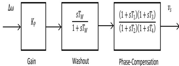
Fig. 1: Block diagram of PSS controlled plant
