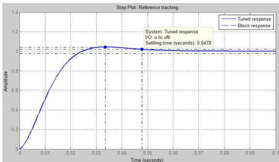
Fig. 17 ICA-PID reference tracking on time graph
