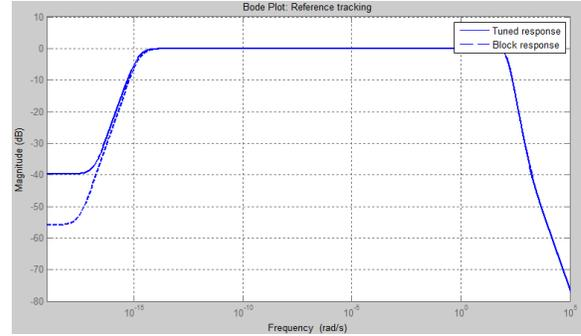
Fig. 18 ICA-PID reference tracking on frequency graph
