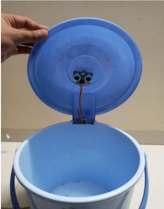
Fig.5. HC-SR04 Ultrasonic Sensor attached to dustbin
