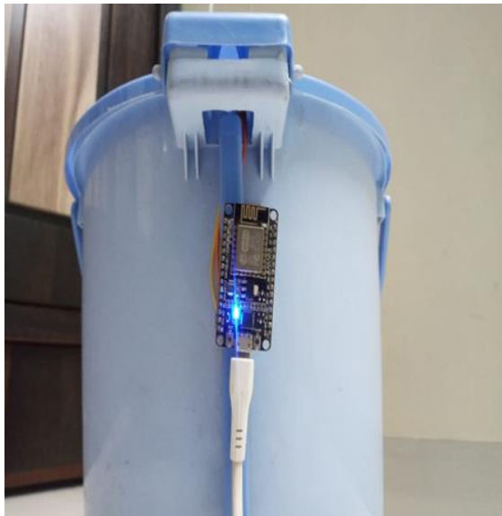
Fig.6. NODEMCU ESP 8266 Wi-Fi module attached to exterior side of dustbin
