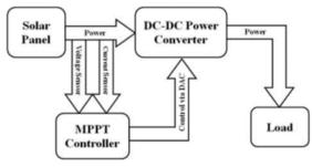
Fig 1: Block diagram of MPPT
