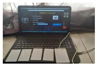
Figure 10. A picture showing the RFID tag and reader been Used
