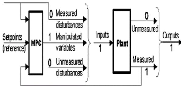
Fig. 9 Structure of the designed MPC in MATLAB/Simulink
