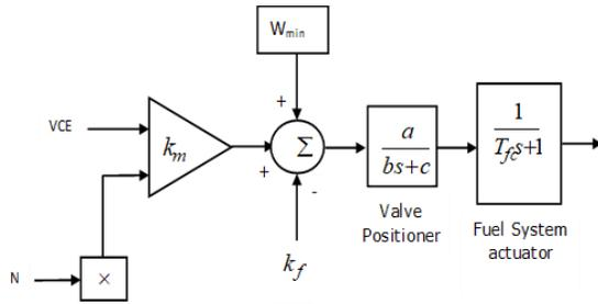
Fig. 6 Simulink block of the fuel system
