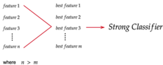
Figure4: The AdaBoost algorithm's purpose is to extract the best features from a set of n features.
