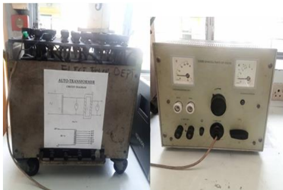
Fig. 13: Laboratory picture of Auto-Transformer Starting Method of a three-phase Squirrel Cage Induction Motor (Electrical Machine Laboratory Rivers State University 2020)
