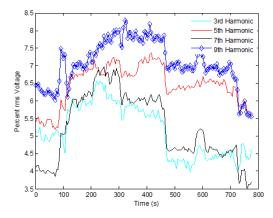
Fig. 6: Comparison of Dominant Harmonic Components with all Loads Connected
