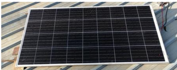
Figure.3 Front view of solar photovoltaic thermal collector
