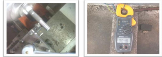
Figure 3.3 The process of turning and measuring the current of an electric motor
