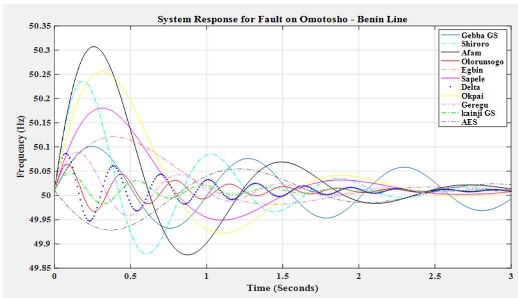
Figure 10: Frequency response of the system generators for fault clearing time of 0.3sec (with only VSC-HVDC)
