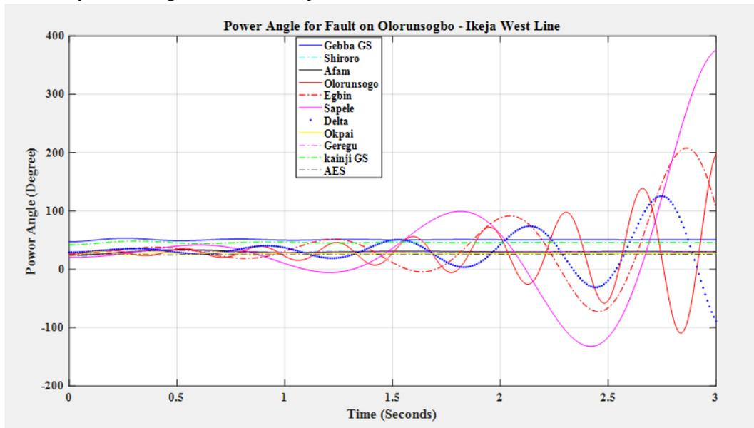
Figure 3: Power Angle response of the generators for fault clearing time of 0.3sec (without any VSC-HVDC)
