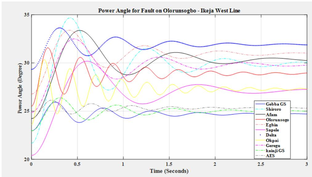
Figure 7: Power Angle response of the generators for fault clearing time of 0.3sec (with only VSC-HVDC)
