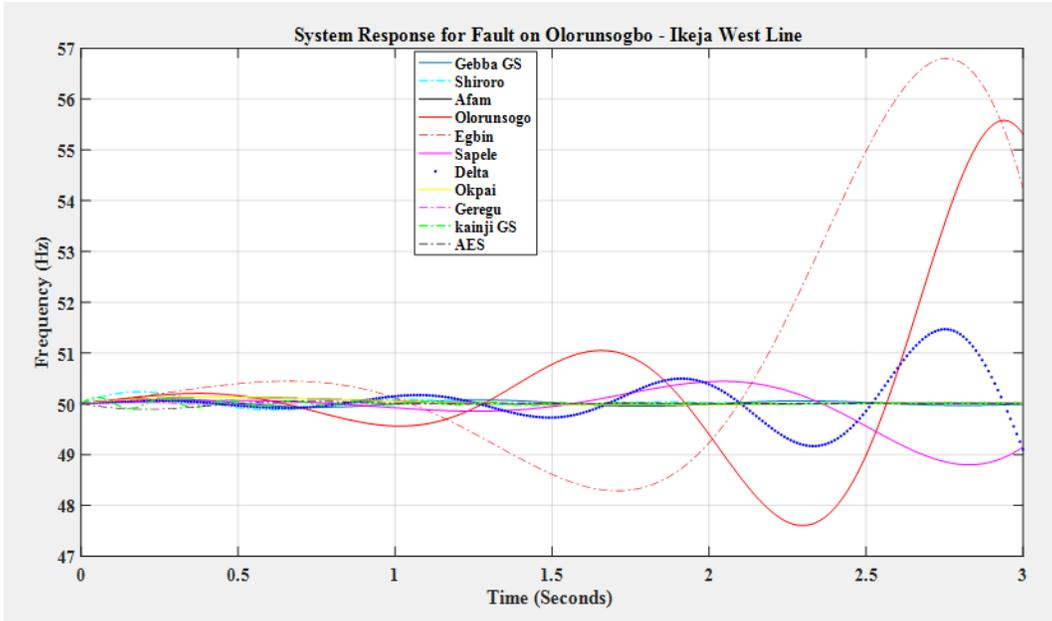
Figure 4: Frequency response of the system generators for fault clearing time of 0.3sec (without any VSC-HVDC)
