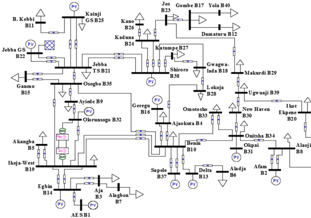
Figure 1: PSAT Model of the Nigeria 330kV transmission power system with VSC-HVDC installed along side with Olorunsogbo – Ikeja West Transmission Line
