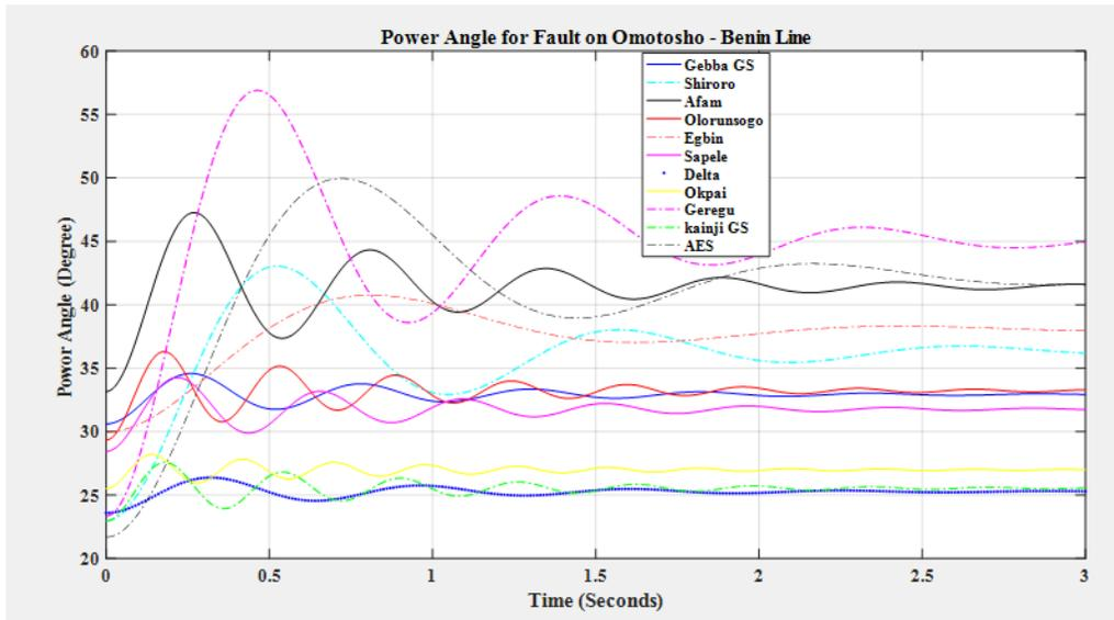
Figure 9: Power Angle response of the generators for fault clearing time of 0.3sec (with only VSC-HVDC)
