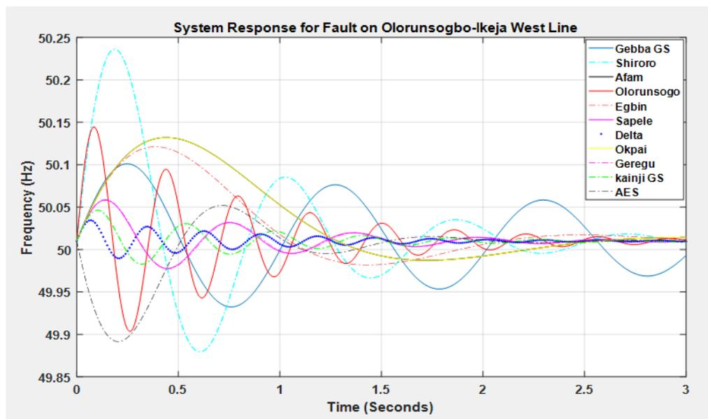
Figure 8: Frequency response of the system generators for fault clearing time of 0.3sec (with only VSC-HVDC).
