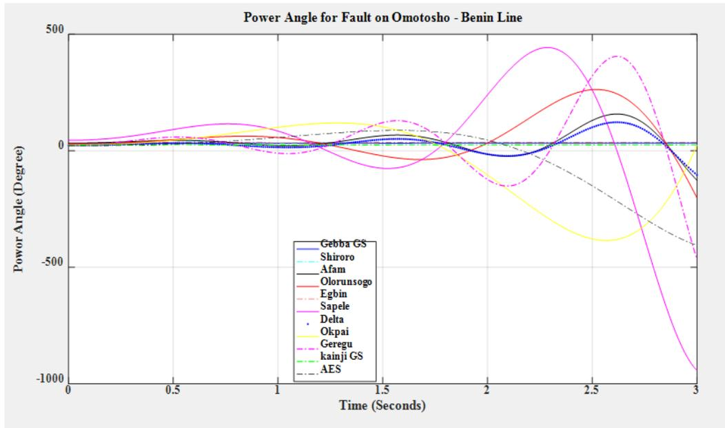
Figure 5: Power Angle response of the generators for fault clearing time of 0.3sec (without any VSC-HVDC)
