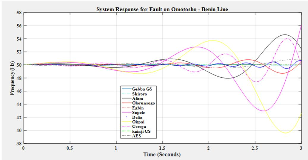
Figure 6: Frequency response of the system generators for fault clearing time of 0.3sec (without any VSC-HVDC)
