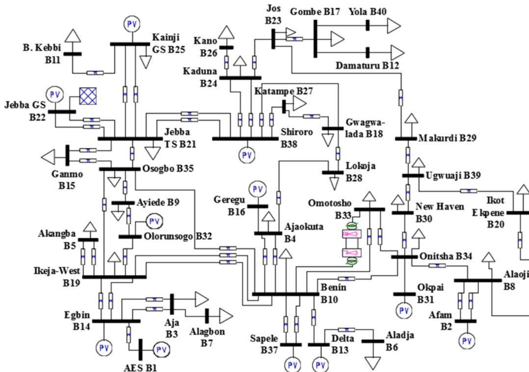
Figure 2: PSAT Model of the Nigeria 330kV transmission power system with VSC-HVDC installed along side with Omotosho – Benin Transmission Line
