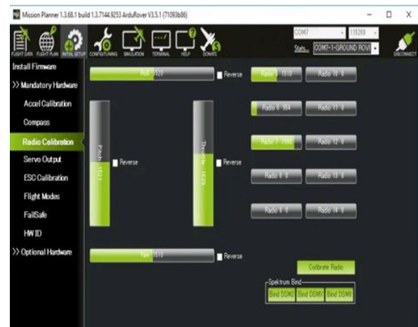
Figure 11: Calibration of the Radio Transmitter
