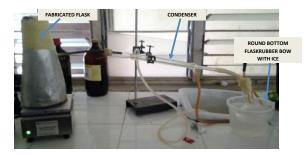
Figure 3.3: Steam Distillation
