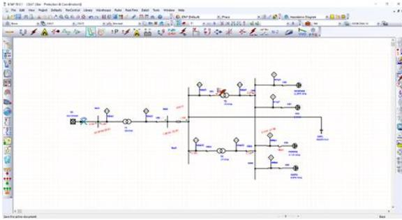
Figure-5: Relay Coordination Scheme in RSU
