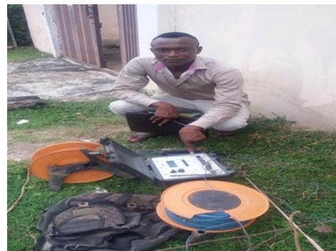
Figure 3: Picture of an Omega resistivity meter, electric cables and electrodes.
