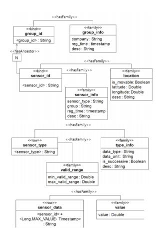
Figure 1. Sensor data schema
