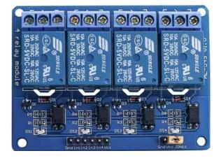
A relay is an electrical device which is generally used to control high voltages using very low voltage as an 35 Input. This consists of a coil wrapped around a pole
