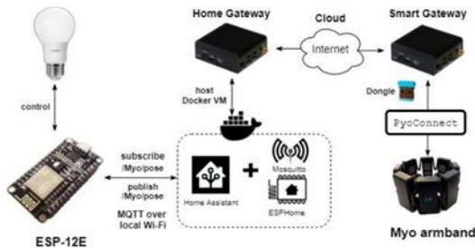
Fig: The presented EMG-based IoT system architecture
