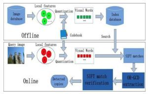
Fig. 4. The framework of our copy detection method.
