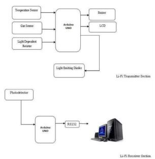
Fig.4: Block Diagram of Proposed System
