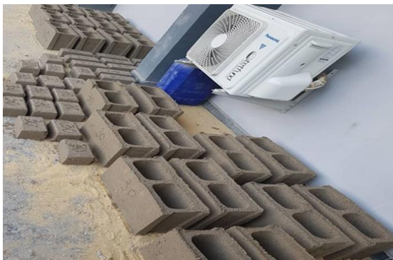
Fig 2: Removal of sand-crete hollow blocks on a clean surface
