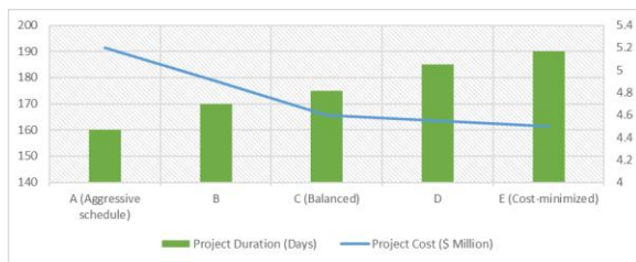
Figure 4: Trade-Off Curve — Project Cost vs. Duration
