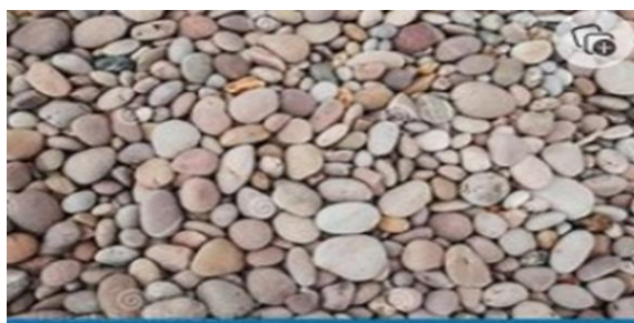
Assorted natural rock pebbles that are commonly used as thermal energy storage materials due to their availability and high thermal mass
