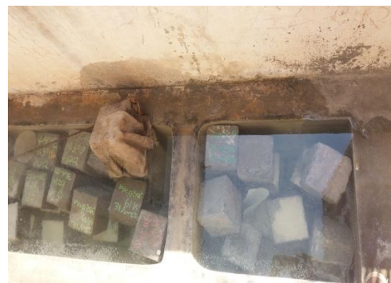
Fig No.6 Curing Of Cubes in Curing Tank
