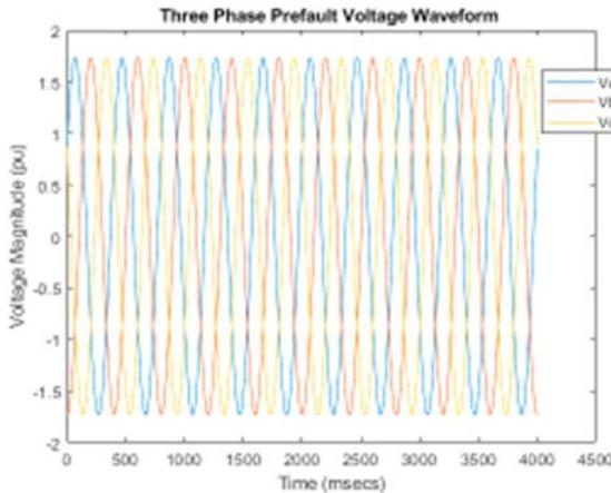
Figure 2: Three Phase Pre-fault Voltage Waveform
