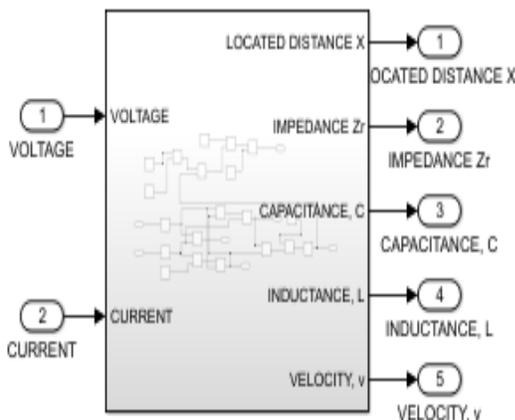
Figure 9: Subsystem of Traveling Wave Fault Location Model
