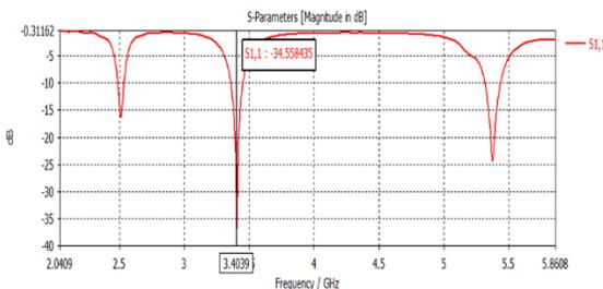
Figure 7: Simulation Return Loss Graph For Bending Antenna
