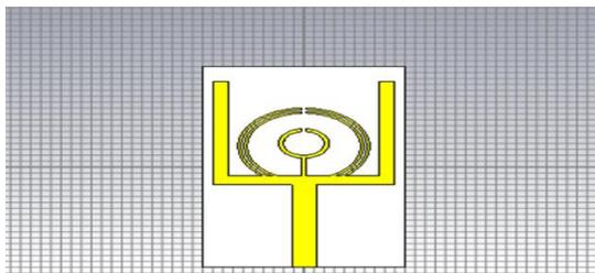
Figure 2: Proposed Antenna without bending
