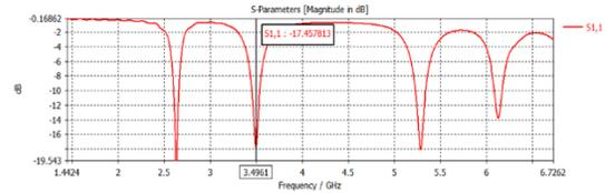
Figure 3: Simulation Return Loss Graph
