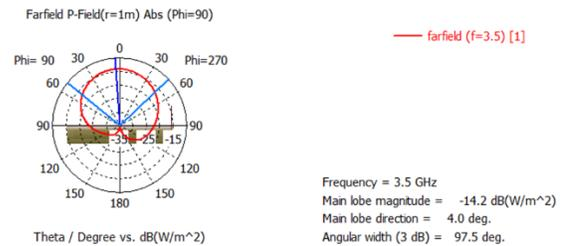
Figure 9: Radiation pattern For Bending Antenna
