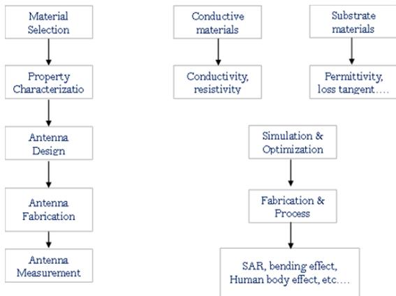
Figure: 1 Design flow procedure
