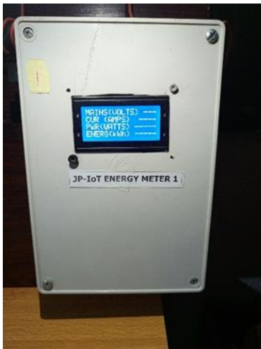
Figure 9. Energy meter display during no load test with hotspot off
