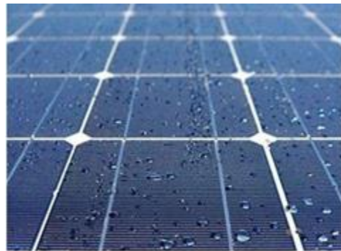
Picture of a hydrophobic treated panel where water accumulates into droplets for easy roll down
