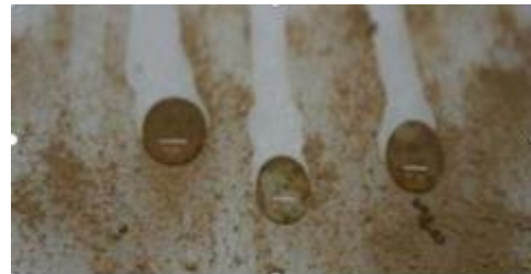
Picture depicting self-cleaning & rolling down of water droplets Carrying dust particles on a hydrophobic surface
