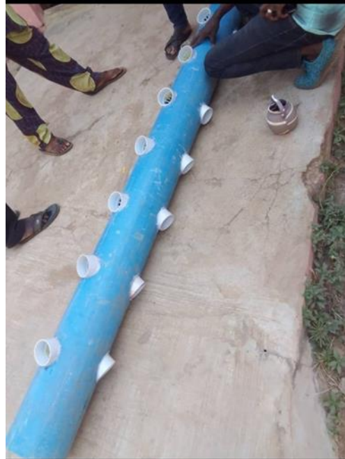
Figure 5: Fixing of the plant cups on the bored PVC pipes
