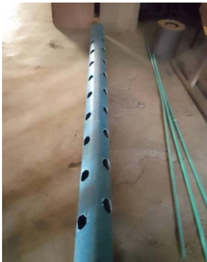
Figure 4: Bored PVC pipes with 28 numbers 10 cm elliptical holes
