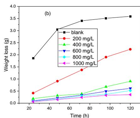
Figure 2 Weight loss vs time for mild steel corrosion in (a) 1 M HCl and (b) 0.5 M H<sub>2</sub>SO<sub>4</sub> in the absence and presence of different concentrations of DH
