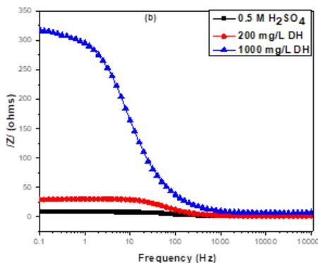
Figure 5. Electrochemical impedance spectra of mild steel in 0.5 M  $\text{H}_2\text{SO}_4$  solution without and with DH extract: (a) Nyquist and (b) Bode plots. Inset in panel (a) is the Nyquist plot in uninhibited acid.
