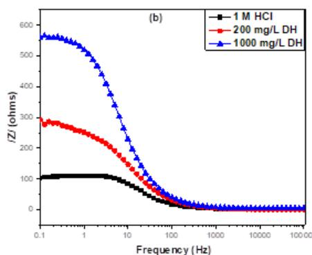
Figure 4. Electrochemical impedance spectra of mild steel in 1 M HCl solution without and with DH extract: (a) Nyquist and (b) Bode plot
