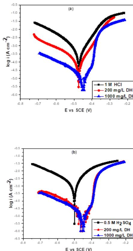
Figure 6. Potentiodynamic polarization curves of mild steel in (a) 1 M HCl and (b) 0.5 M H<sub>2</sub>SO<sub>4</sub> solution without and with DH extract.
