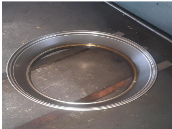
Fig 9: 30 × 1 Inch Connector Showing Top and Bottom Seal
