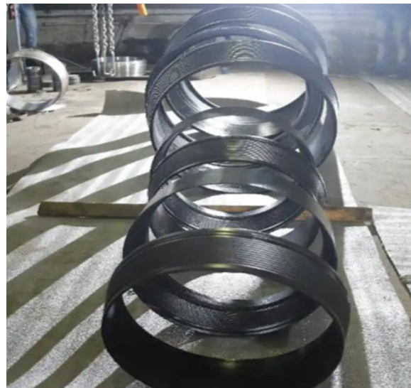
Fig 7: Threaded 30 × 1 Inch PIN Casing Connector after the Threading Process.
