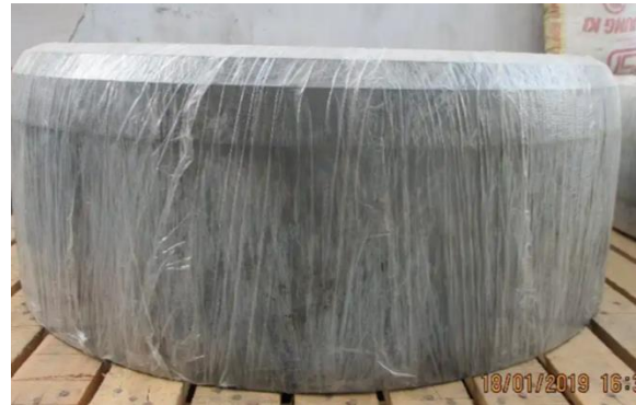
Fig 5: Raw Casing connector Material for Machining
