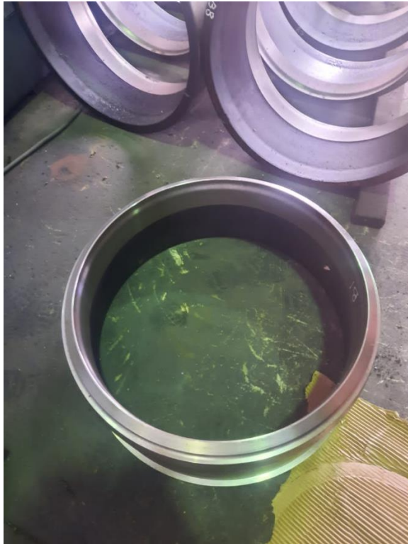
Fig.6: 30 × 1 Inch Connector with Weld Prep after Blanking.
