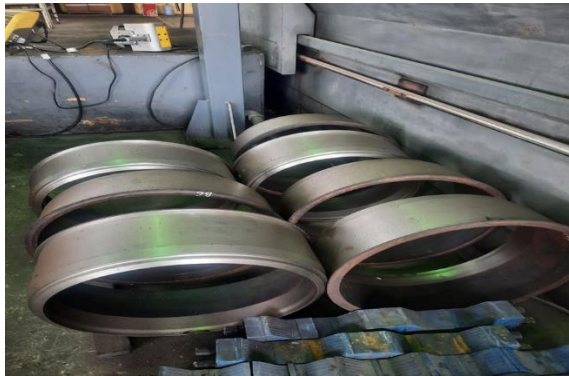
Fig 8: Blanking of the 30 × 1 Inch Casing Connector
