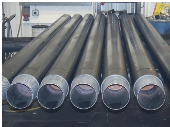
Fig.11: Threaded PIN Connector Welded to Pipe Casing
