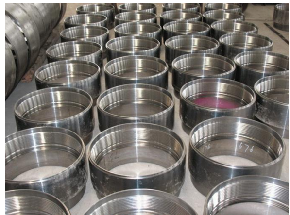
Fig 10: Threaded 30 × 1 Inch BOX Casing Connector after the Threading Process.
