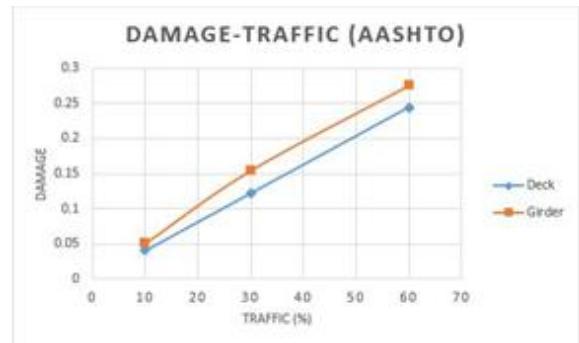
Fig. 14: Bridge Superstructure Damage
