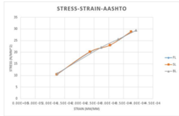
Fig. 13: Bridge Superstructure Stress–Strain
