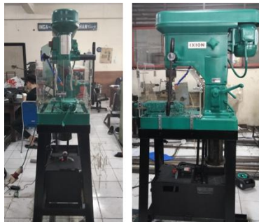
Figure 3.2 IXION BT 25 Bench Drill Machine Cooling System
