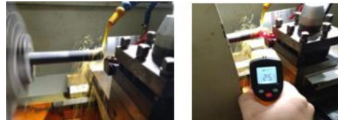
Figure 2.3 Turning Process of Test Objects and Temperature Measurement [4]
