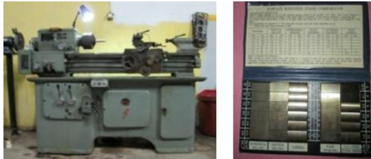
Figure 2.1 Kiangsi Lathe Machine Tool Works Engine Lathe C6127a and Surface Rouness stand Comparator [2]
