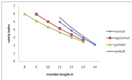
Fig. 2: Variation of  $\beta$  with the span, L (UDL in bending)
