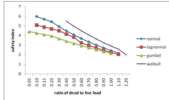
Fig. 8: Variation of  $\beta$  with ratio of dead load to live load,  $g/q$  (UDL shear)
