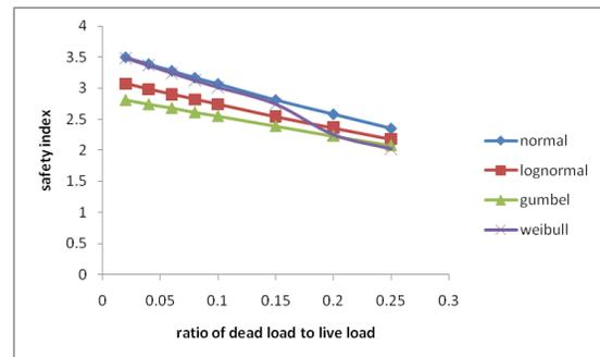
Fig. 9: Variation of  $\beta$  with ratio of dead load to live load,  $G/Q$  (point load in bending)
