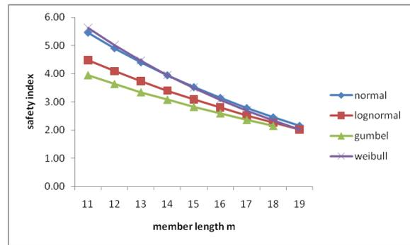
Fig. 4: Variation of  $\beta$  with span, L (Point load in bending)
