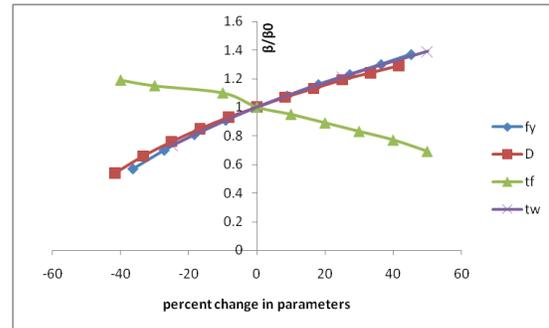
Fig. 14: Sensitivity plots for shear consideration under uniformly distributed load
