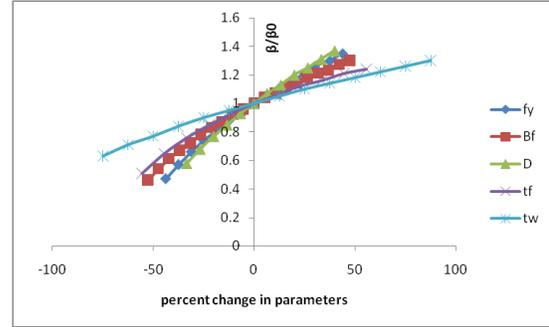
Fig. 13: Sensitivity plots for bending consideration under uniformly distributed load
