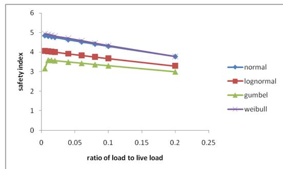
Fig. 10: Variation of  $\beta$  with ratio of dead load to live load,  $G/Q$  (point load in shear)
