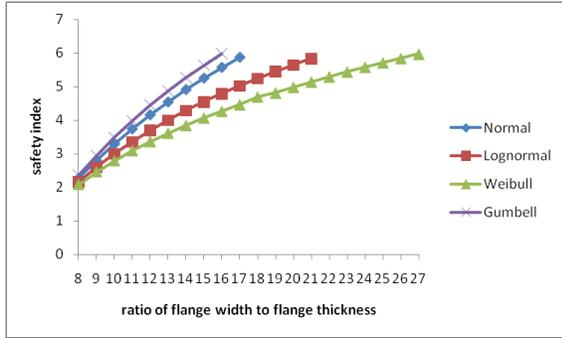
Fig. 11: Variation of  $\beta$  with the ratio of flange width to thickness,  $B_f/t_f$  (UDL in bending)
