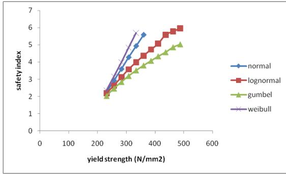
Fig. 5: Variation of  $\beta$  with yield strength,  $f_y$  (UDL in bending)
