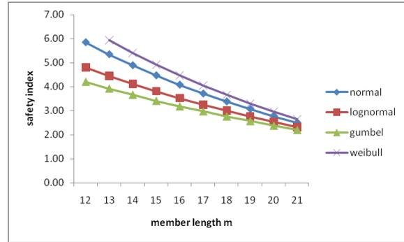
Fig. 3: Variation of  $\beta$  with the span, L (UDL in shear)
