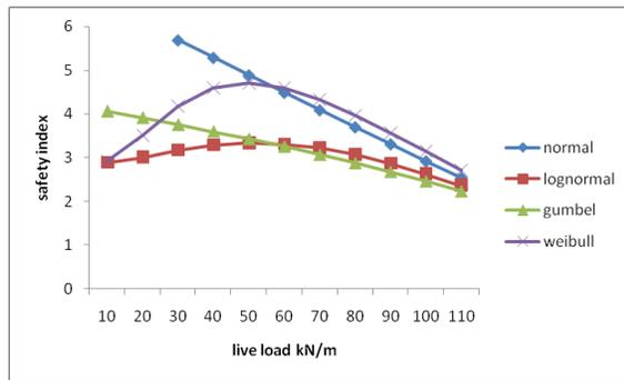
Fig. 6: Variation of  $\beta$  with live load,  $q$  (UDL in bending)
