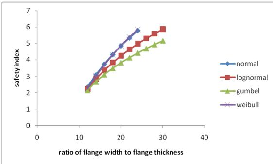
Fig. 12: Variation of  $\beta$  with the ratio of flange width to thickness,  $B_f/t_f$  (Point load in bending)
