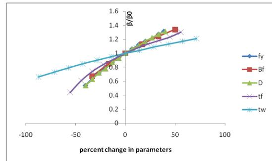
Fig. 15: Sensitivity plots for bending consideration under point load.
