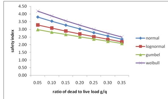
Fig. 7: Variation of  $\beta$  with ratio of dead load to live load,  $g/q$  (UDL bending)
