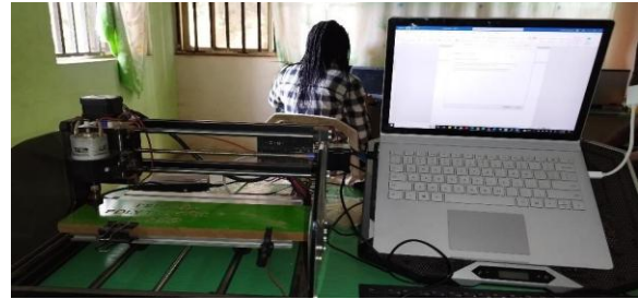
Figure 3: The CNC milling machine with computer controller screen window
