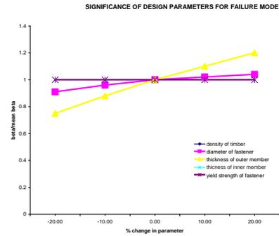
Fig. 24: Sensitivity Plot for Failure Mode I
