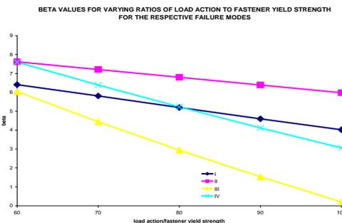
Fig. 19: Variation of  $\beta$  with ratios of load action to the fastener yield strength.
