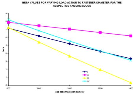
Fig. 16: Variation of  $\beta$  with ratios of load action to fastener diameter.
