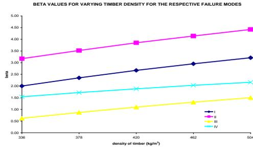
Fig. 4: Variation of  $\beta$  with density of timber.
