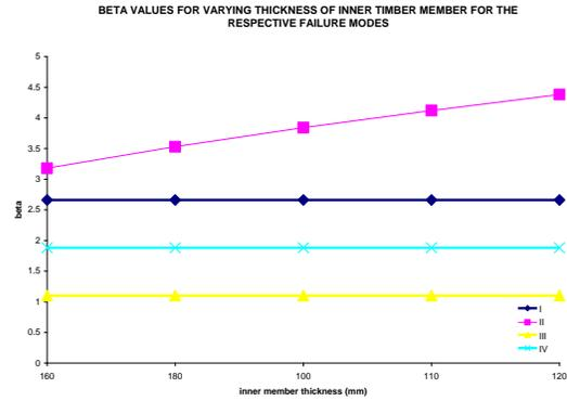
Fig. 7: Variation of  $\beta$  with thickness of inner member.
