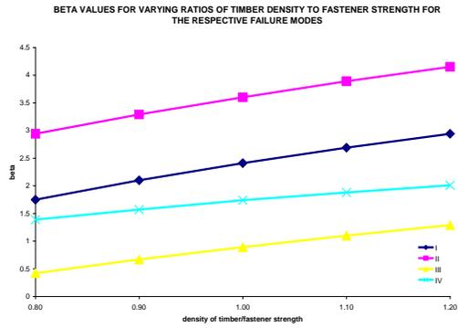
Fig. 10: Variation of  $\beta$  with ratios of timber density to fastener yield strength.
