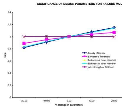
Fig. 25: Sensitivity Plot for Failure Mode II
