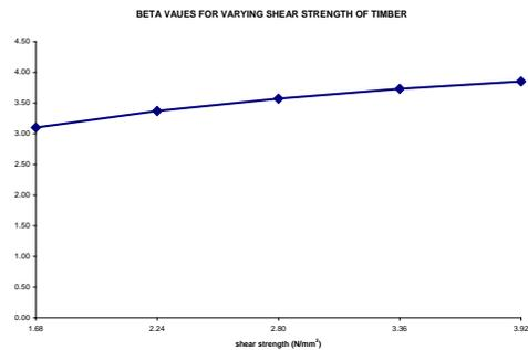
Fig. 20: Variation of  $\beta$  with shear strength of timber for shear consideration.
