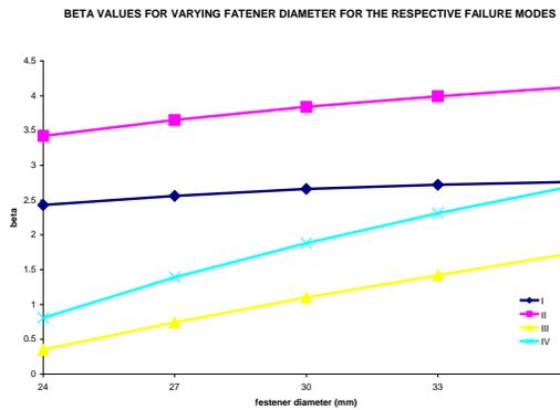
Fig. 5: Variation of  $\beta$  with diameter of fastener.
