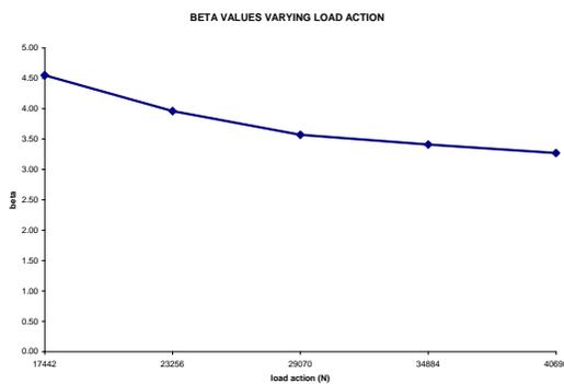
Fig. 23: Variation of  $\beta$  with the resultant load action for shear consideration.
