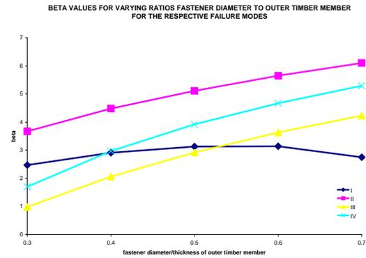
Fig. 13: Variation of  $\beta$  with ratios of fastener diameter to the thickness of outer member of timber.
