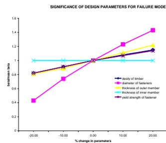
Fig. 27: Sensitivity Plot for Failure Mode IV
