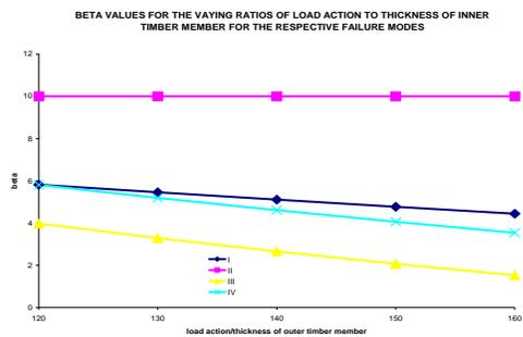
Fig. 18: Variation of  $\beta$  with ratios of load action to the thickness of inner member of timber.
