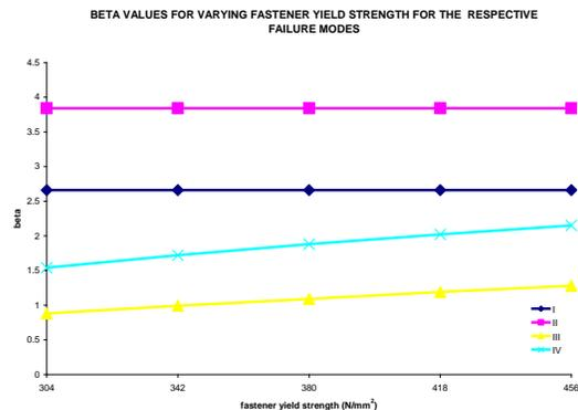
Fig. 9: Variation of  $\beta$  with yield strength of fastener.
