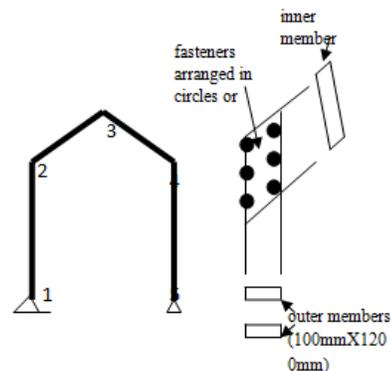
Figure 3: Geometry of the frame and outline of the knee joint
