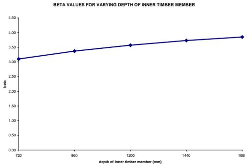
Fig. 22: Variation of  $\beta$  with the thickness of inner member of timber for shear consideration.
