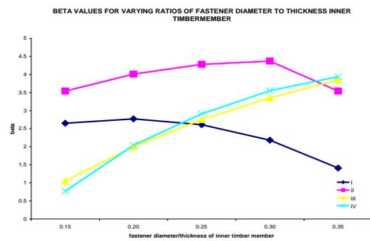
Fig. 14: Variation of  $\beta$  with ratios of fastener diameter to the thickness of inner member of timber.
