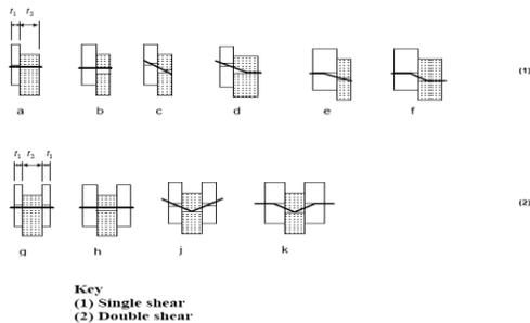
Fig. 2: Failure modes for dowel-type timber joints.
