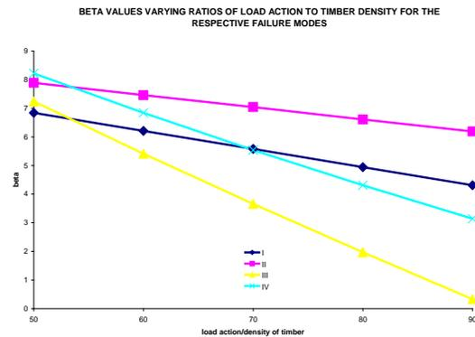
Fig. 15: Variation of  $\beta$  with ratios of load action to timber density.
