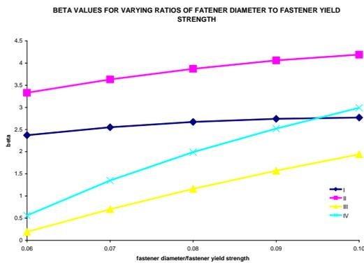
Fig. 12: Variation of  $\beta$  with ratios of fastener diameter to fastener yield strength.
