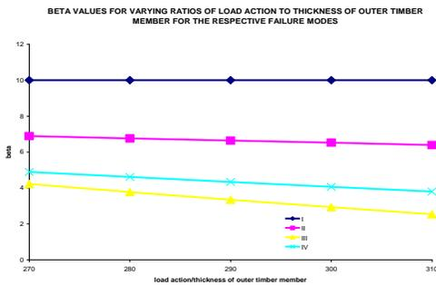
Fig. 17: Variation of  $\beta$  with ratios of load action to the thickness of outer member of timber.
