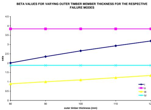
Fig. 6: Variation of  $\beta$  with thickness of outer member.
