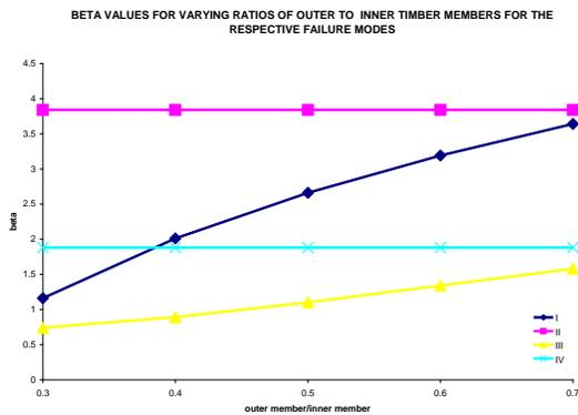
Fig. 11: Variation of  $\beta$  with ratios of thickness of outer to inner member.
