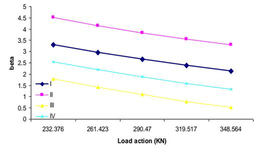
Fig. 8: Variation of  $\beta$  with resultant load action.
