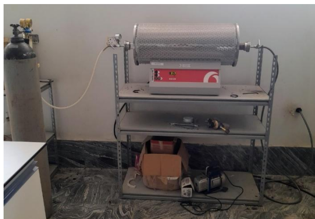
Plate III: Chemical Vapor Deposition Apparatus used for the Pyrolysis
