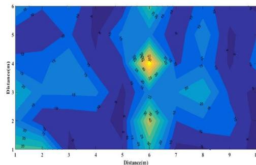
Fig. 3.6: Contour plot of the magnetic flux density at a height of 1m
