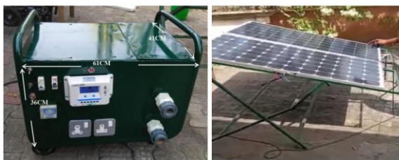
Figure 2: Isometric View of the Mobile Standalone Solar Powered Water Pumping System
