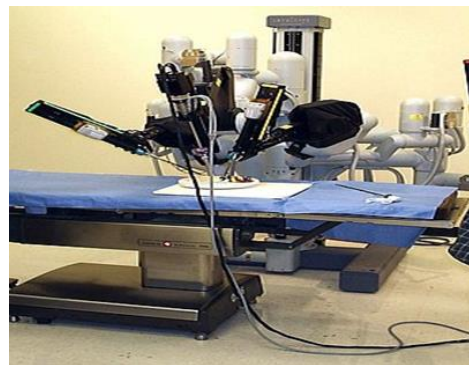
Figure 1: A robotically assisted surgical system used for prostatectomies, cardiac valve repair and gynecologic surgical procedures
