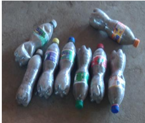
Figure 3: Empty waste PET bottles and those filled with sand.
