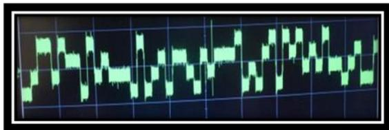
Figure 3.0: 4 level output of convolutional encoder with 14 dB noise
