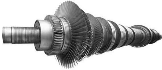
Figure 7. Steam Turbine Rotor
