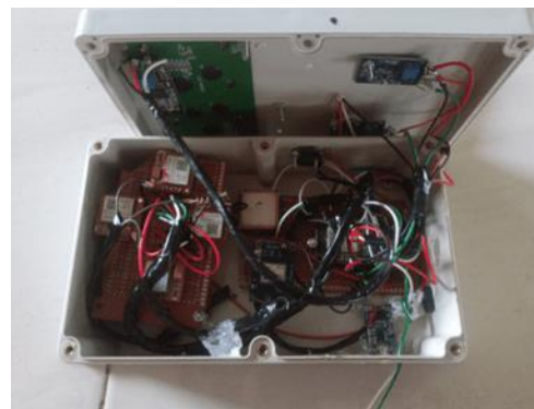
Plate 3: Internal Circuitry of GSS-MPD
