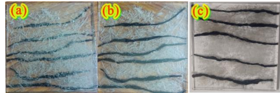
Fig.2 (a) Sample 1 - 10% human hair and 30% chicken feather, (b) Sample 2 - 20% human hair and 20% chicken feather, (c) Sample 3 - 30% human hair and 10% chicken feather.
