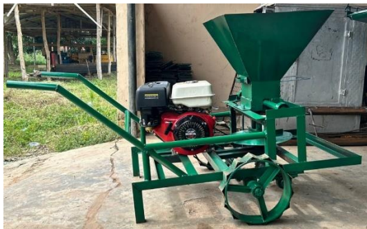
Fig 4: Photograph of the fabricated manure spreader
