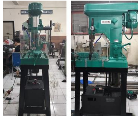
Figure 2.2 Cooling System Design Results on the IXION BT 25 Bench Drill Machine [7]
